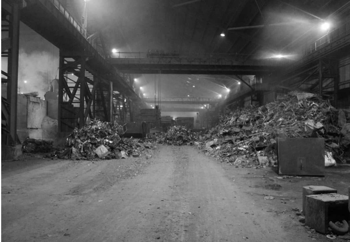
Figure 18. Scrap is broken into small pieces and placed near the blast furnaces
