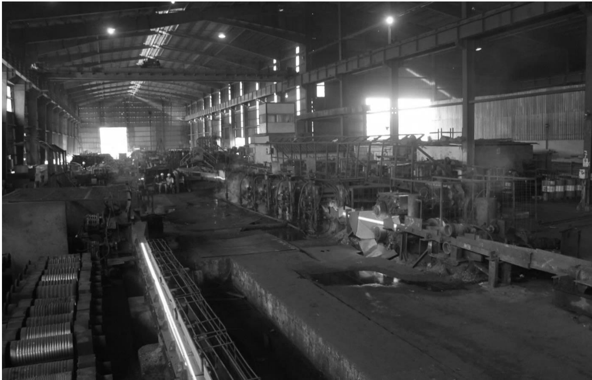
Figure 21. The rolling stand through which hot iron is passed
