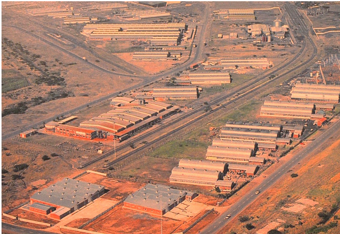
FIGURE 5.2: Aerial view of an RIDP site in Zone E (Itsetebe). The image demonstrates a typical RIDP site built between railway lines with sidings servicing each arm of the complex. As the complexes were expanded, additional railway sidings could be added.
